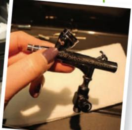
We then watched how to take all of the gun's components apart for the deep clean that's necessary in between use, so the gun doesn't get clogged up. Starting from the back, each mini component got a thorough clean before we put it all back together – and I was warned that it would be difficult to do with long nails!
