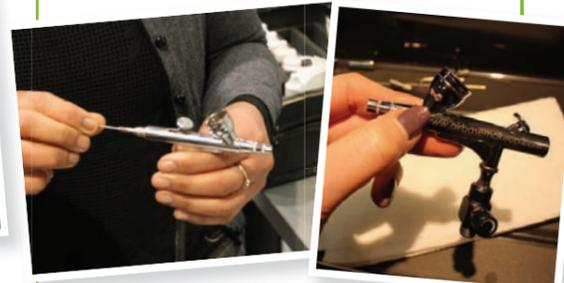
We then watched how to take all of the gun's components apart for the deep clean that's necessary in between use, so the gun doesn't get clogged up. Starting from the back, each mini component got a thorough clean before we put it all back together – and I was warned that it would be difficult to do with long nails!
